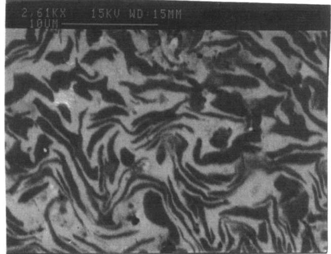
Fig. 6. Microstructure of deformation processed titanium–50 vol.% yttrium.
